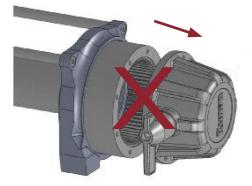
**Step 2** Rotate the gearbox anti-clockwise.
